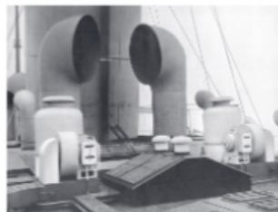
Top, is a 'top suction deck type' as fitted on the SS Heliopolis of 1907.
