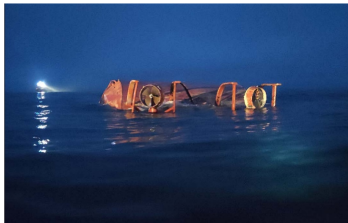
Karin Hoj's upturned hull, showing azimuth drive units at the stern.
